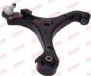
https://ikoyama.com/img/T1228.png HONDA CIVIC 11/14 TRAPECIO DEL IZQ 51350-TR0-A01
