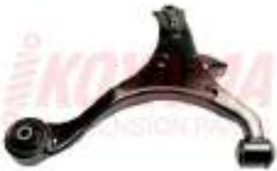
https://ikoyama.com/img/T1174.png HONDA CIVIC 01/05 TRAPECIO DEL IZQ 51360-S5A-A03
