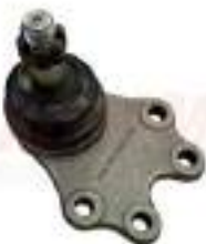
https://ikoyama.com/img/RT0008.png TOYOTA HIACE CONMUTER 3L 90/95 ROTULA DEL SUP RH LH 43350-29065 CBT-34
